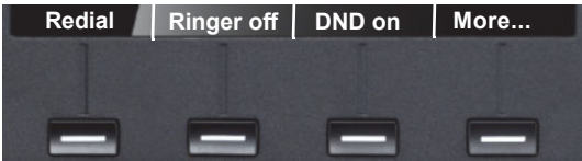
The OpenScapeDesk Phone IP 55G has four Soft Keys providing context sensitive features. The "More..." Soft Key (if shown) provides access to more options.
